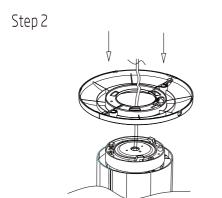
2.Position the base on the bottom of the fan, put the power cord through the base and make sure clasps on tower fan body is align with the holes on the base. See step 2.
