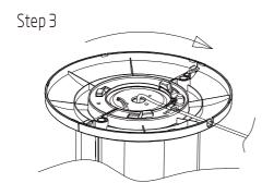
3. Then rotate the base clockwise until the it is locked. Finally thread the power cord into the guide on the bottom of the base by gently pressing the wire into the clamps. See step 3.
