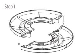
1. Put the two halves of the base together. See step 1.
